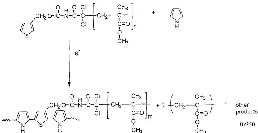
**SCHEME 2** Mechanism of electrochemical polymerization of polypyrrole on TPMMA substrate.
