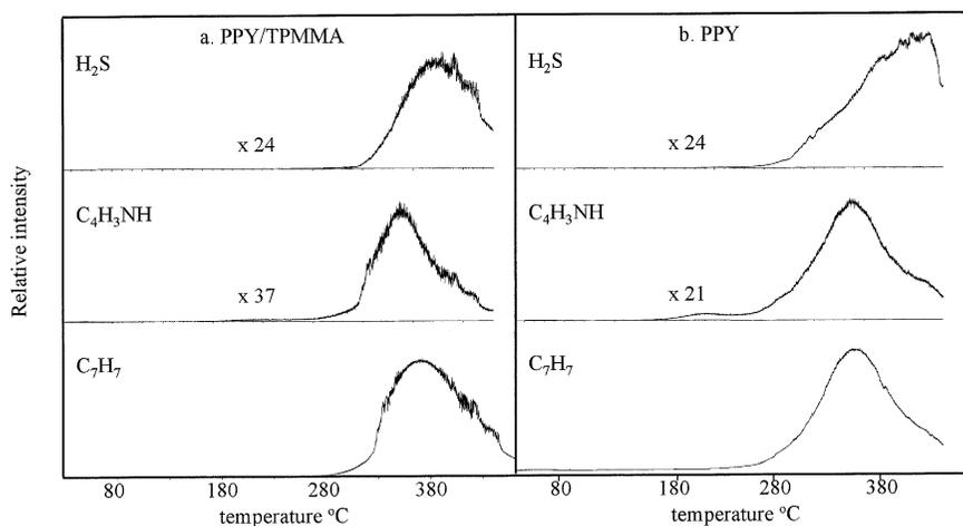
**FIGURE 4** Single ion pyrograms of the fragments at  $m/z$  91 due to  $C_7H_7$ , 66 due to  $C_4H_3NH$ , and 34 due to  $H_2S$  of (a) PPY/TPMMA and (b) PPY.
