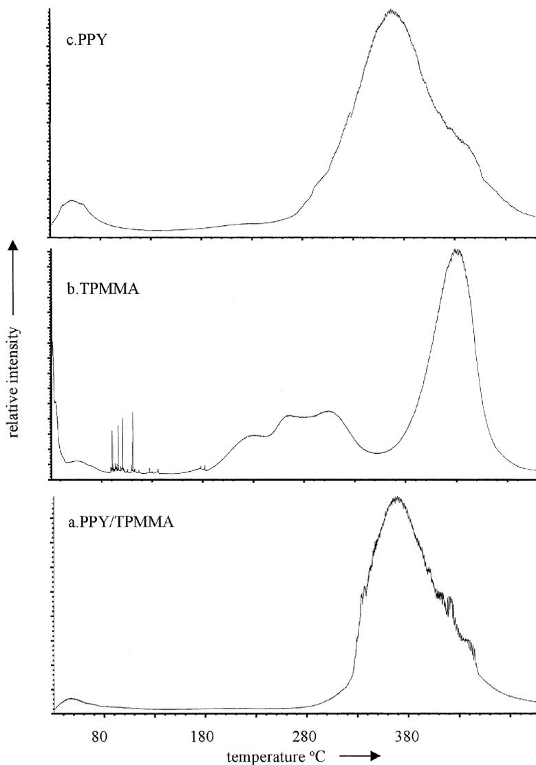
**FIGURE 1** TIC curves of (a) PPY/TPMMA (b) PPY, and (c) TPMMA.
