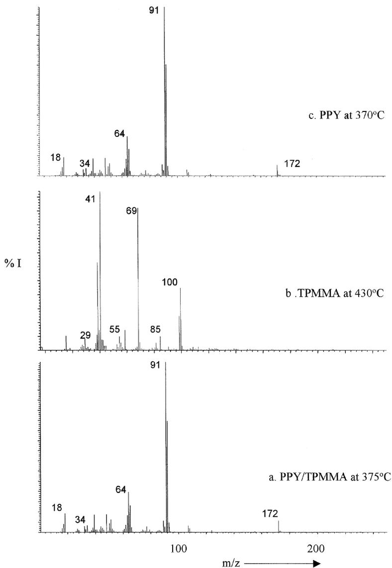
**FIGURE 2** The pyrolysis mass spectra for (a) PPY/TPMMA, (b) PPY, and (c) TPMMA at the maximum of the corresponding TIC curves.
