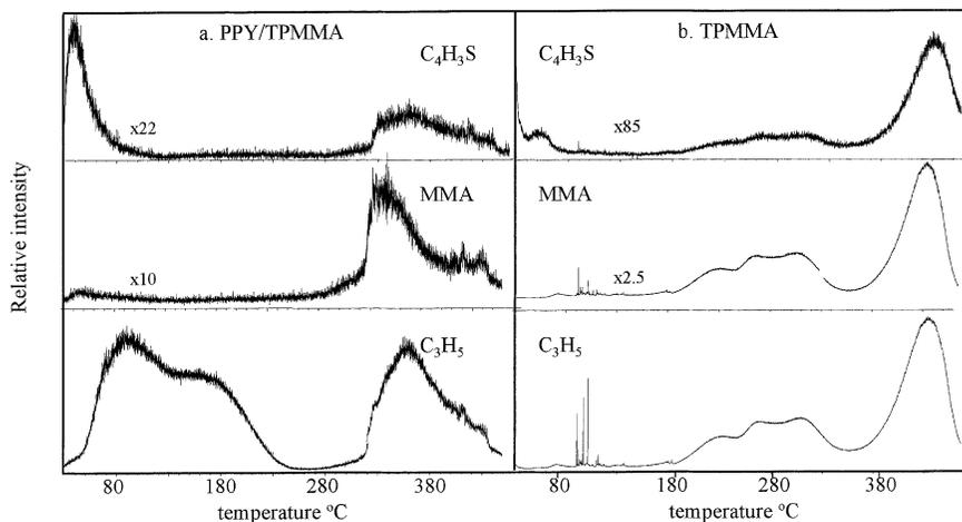
**FIGURE 3** Single ion pyrograms of the fragments at  $m/z$  100 due to MMA, 41 due to  $C_3H_5$  and 83  $C_4H_3S$  of (a) PPY/TPMMA and (b) PPY.
